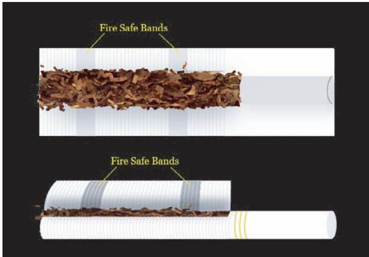
Figure 2.1 Composition of a reduced ignition cigarette
